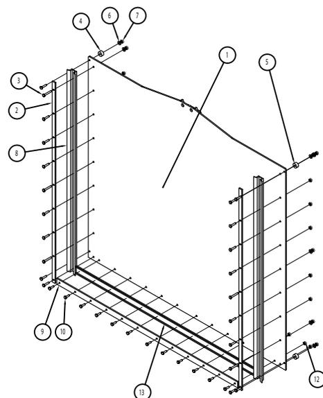
Figure 18: Side seal and bottom seal replacement
