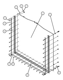
Figure 18: Side seal and bottom seal replacement
