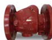
Series 5190/00 Flanged swing check valve Spring loaded Grooved ends to AWWA C606 DN50-200 24,1 bar (300 PSI) UL/ULC listed, FM approved
