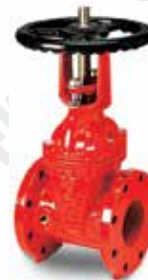
Series 45/56 Flanged gate valve with rising stem DN50-300: 17,2 bar (250 PSI) DN350-400: 13,7 bar (200 PSI) Ductile iron UL/ULC listed, FM approved
